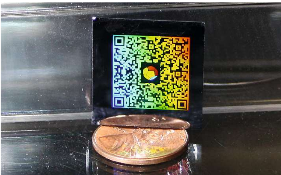
Fig. 1 Example of a colorful QR code consisting of diffractive dot arrays.
